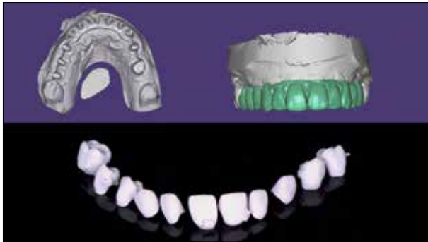
Fig 36 Design and fabrication of twelve individually milled monolithic CAD/CAM ceramic crowns (e.max CAD; Ivoclar Vivadent; lithium disilicate).
